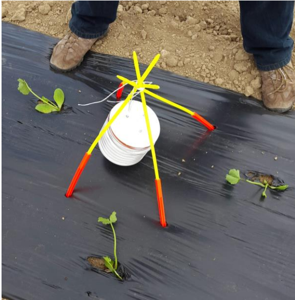
Figure 3. Logger placed in an early courgette crop on the South coast, 2015
